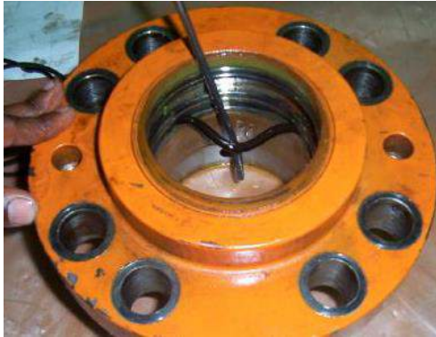
Step-17 Remove the rod seal from head end cover.
