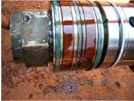
Step 9 Mark the piston rod & piston nut before opening the piston nut. This will ensure the torque while retightening
